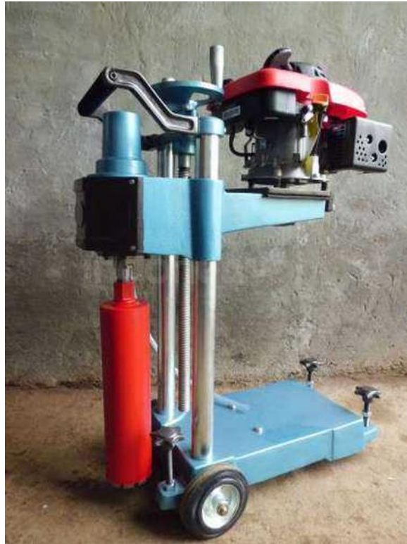
Gambar 3. 6 Core drill Machine
