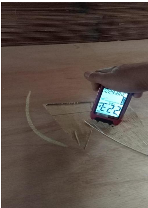
Delaminasi face/back kadar air tinggi
