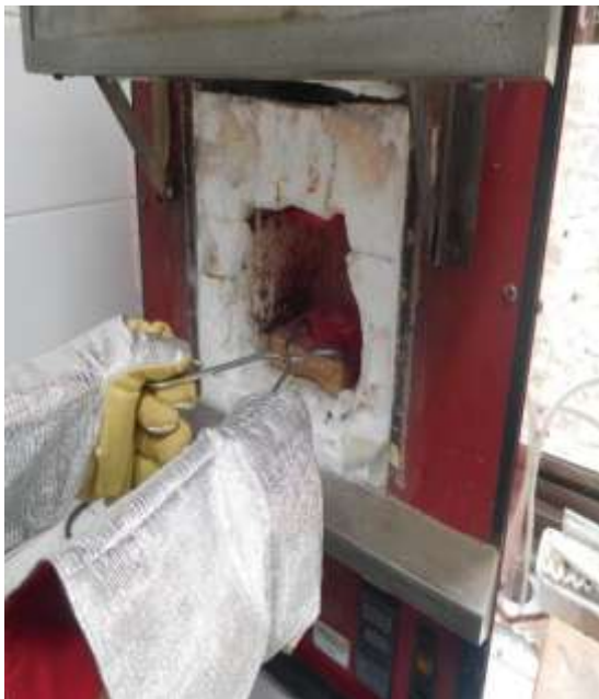
Proses annealing sampel B
