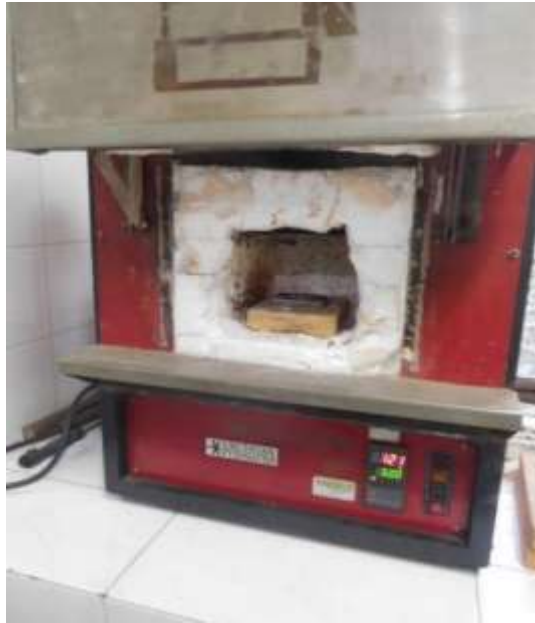
Proses annealing sampel B
